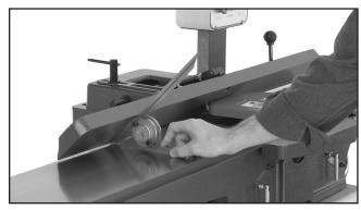
**Figure 62.** Example of adjusting fence 45° inward.
